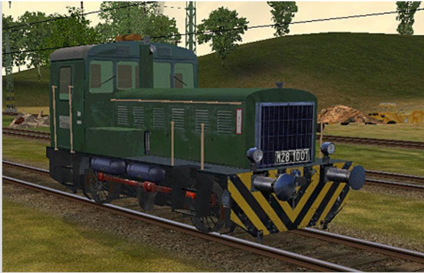
Very small two-axel shunter. Subclass M28.1 has a mechanical transmission and the more powerful M28.2 Hydraulic.
